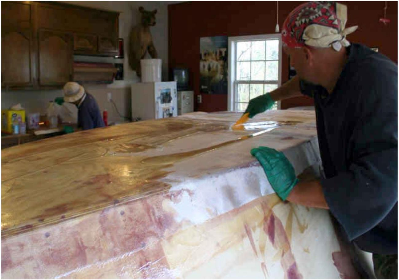
Now the fiberglassing begins. The trick is to only use enough resin to fully saturate the glass cloth without building up excess layers. You can tell when there's enough resin because the opaque cloth disappears and turns transparent. It starts to look like a layer of varnish.
