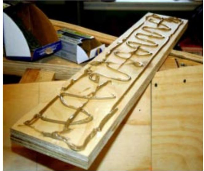
Some designers insist that the plywood joints be scarf jointed together, but this is a precise and complicated process. On Spira International boats, you need only join the plywood using a butt block
