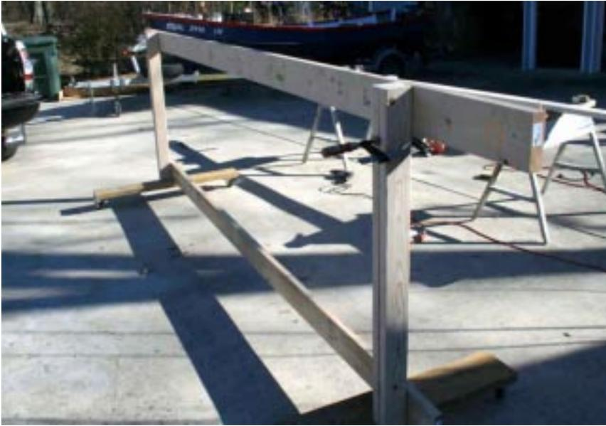
Next, a strongback jig is constructed. This is a sturdy beam on which your boat will be constructed upside down. Some builders elect to put this on wheels so that the project may more easily be rolled into an out of a storage area to make it easier to work on.
