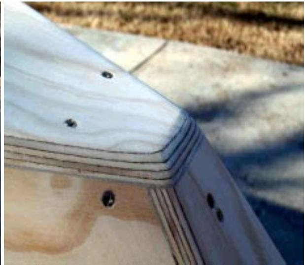
The fully planked hull is sanded smooth and the corners radiused to get ready to fiberglass.
