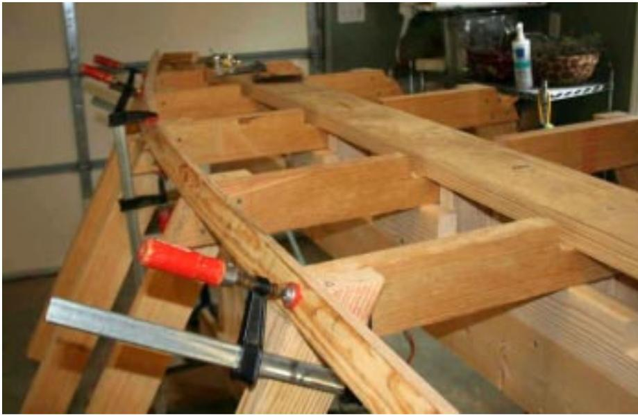
Here the chine log is fitted into the notches in the frames. Once it is fitted in-place, it is glued and screwed in position to form a unitized structure, much stronger than old fashioned wooden boats only held together with screws. In fact, in these boats, you could remove all of the fasteners and it would still be just as strong.
