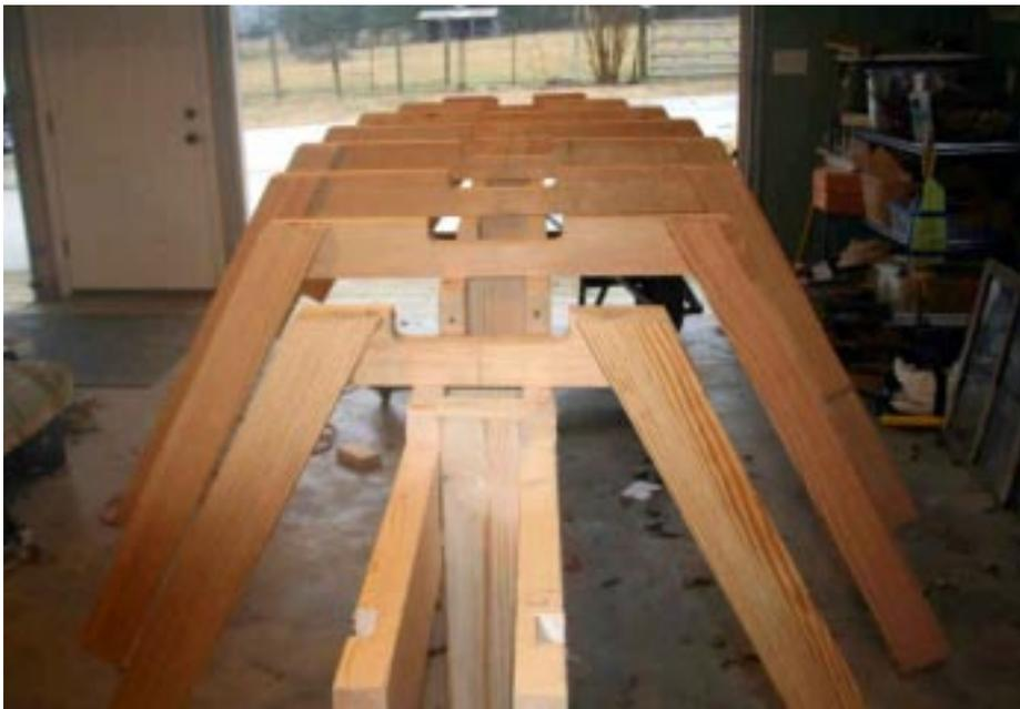
At this stage, everything is squared up to get ready to accept the longitudinal elements. Here you can see the slot for the keelson, cut wider than the actual lumber that makes it up. This leaves space on either side called "Lumber Holes" to allow water to travel between frames and not collect in one spot.
