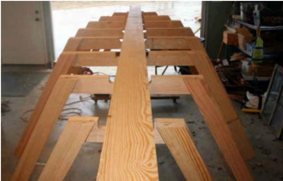
Here the keelson is being fitted to the frames. It is either screwed or bolted to the frames as well as glued using either epoxy or a high-strength, waterproof construction adhesive.
