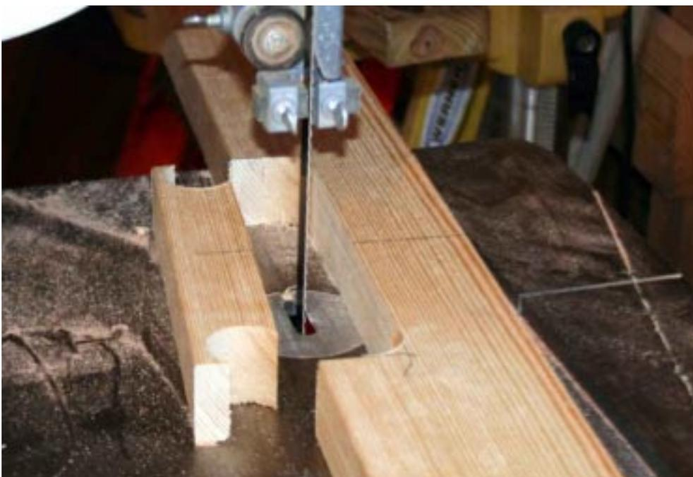
Note how the frames are notched in the center for the keelson to be installed at a later time. A hole is drilled in the corner then the material cut out using a jigsaw or bandsaw. Note also that all frames are straight. There is no need for curves in dory style hull frames, making them very simple to construct.
