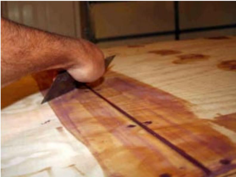
Next you fill the seams and screw holes so that the outside of the hull is smooth and the surface prepared for the fiberglass covering to be added later. The epoxy resin recommended for all Spira International boats, has a strong adhesive property on plywood, unlike the older, less strong polyester resin. There is no need to staple down the fiberglass to the plywood when using epoxy, unlike the methods used for polyester resin fiberglassing.
