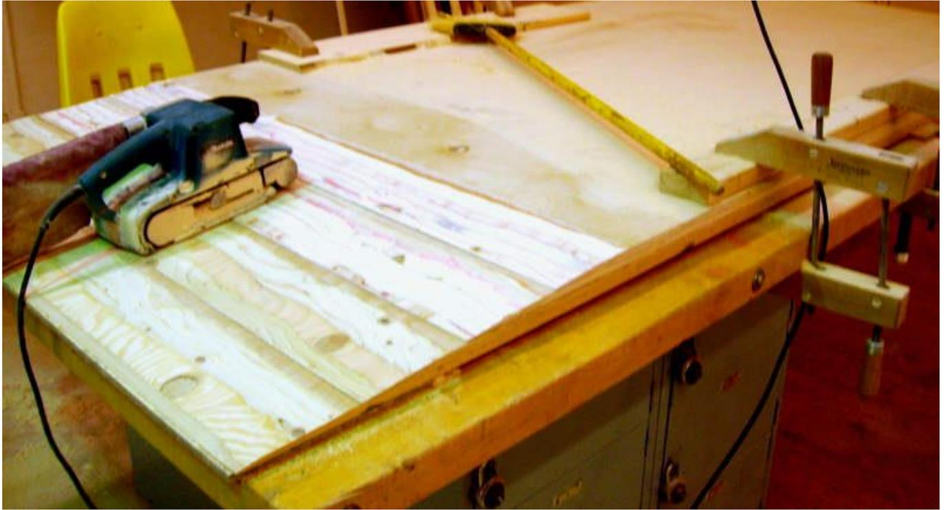
You can also make a simple tool to cut scarfs using a Skill saw. The Gudgeon Brothers used to make a metal one, but I haven't seen one in many years. I don't know if they're still in production, but one of my customers made one from wood that is just as effective as the commercially made one:
